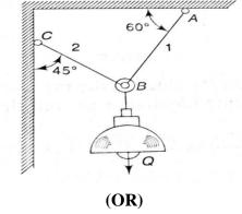
2. a) Tension in cable BC is 725 N. Determine the resultant of forces exerted at point B 6M of beam AB.
