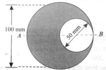
b) Find the moment of inertia of a hollow section shown about horizontal centroidal 6M axis.
